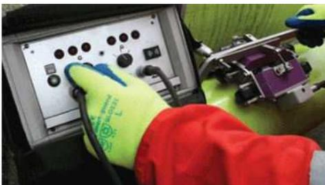
MFL technology can also be employed for rapid inspection of piping looking for general wall reduction.
