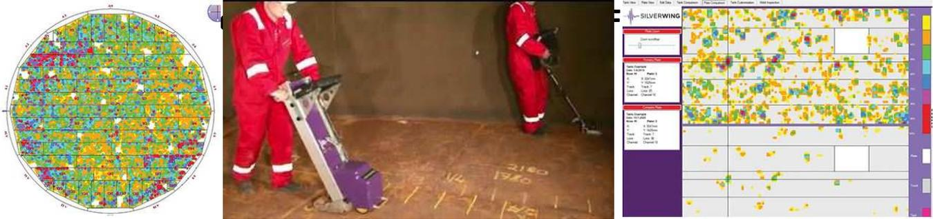
LBI Quality inspection services and Advanced Ultrasonics offers Silverwing Computerised MFL Floormap 3D scanner with STARS technology to provide discrimination between top and bottom surface defects.
